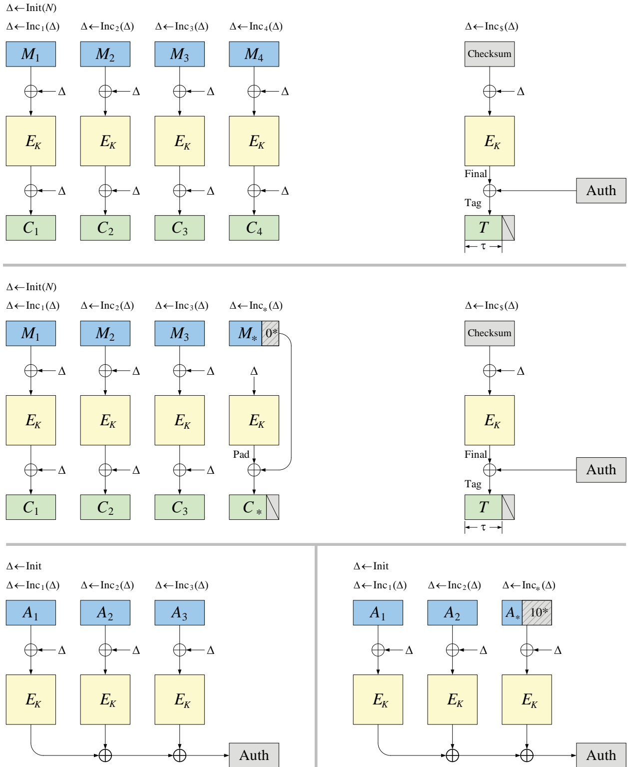
Figure 5: Illustration of OCB3 [E, \tau] . Again E: \mathcal{K} \times \{0, 1\}^{128} \rightarrow \{0, 1\}^n and \tau \in [0..128] . Top: Message M has a full final block ( |M_4| = n ) (Checksum = M_1 \oplus M_2 \oplus M_3 \oplus M_4 ). Middle: Message M has a short final block, 1 \leq |M_*| < n (Checksum = M_1 \oplus M_2 \oplus M_3 \oplus M_* 10^* ). Bottom: An AD of three full blocks (left) or two full blocks and one short one (right). Throughout: Offsets (the \Delta -values) are updated and used top-to-bottom, then left-to-right. Offset initialization and update functions (Init, Inc _i , Inc _s , Inc _* ) return n -bit strings. Each flavor of increment is an xor with some precomputed, K -dependent value.
